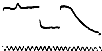
Fig. 9. Radiation from a quartz sandwich experiment done on a 2024 base plate. The radiation begins when the shock enters the first fused quartz plate and decreases when it enters the crystal plate and rises again when it enters the fused quartz cover plate. Relative intensities as well as shock velocities are measured.
